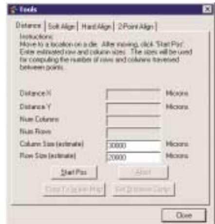
You can quickly measure die sizes using the distance tool.
