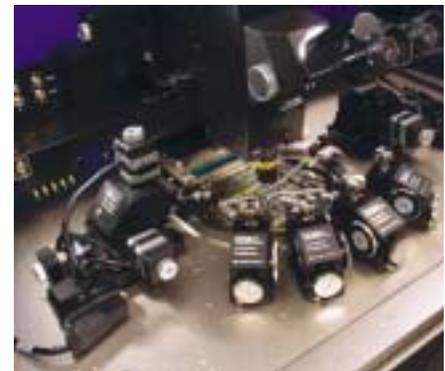
MS1-8 programmable micropositioners enable precision submicron hands-off probing as well as automated step and repeat sub-die testing.
