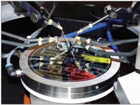
MEMS testing on PM8 with pressure chuck.
