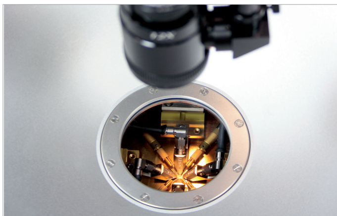
View through the view port of the chamber lid. The shown configuration consists of four RF IZI Probes® and four DC probes.
